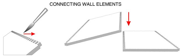
Recommended way of gluing parts together is to apply PVA glue to the interlocking bricks working from back of the part to the front. This ensures there will be no glue overflow on the front, visible side.
